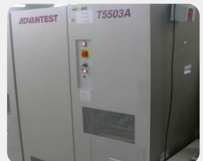
Wide-Temp. IC Sorting via Automatic Test Equipment (ATE)
