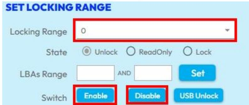
The screenshot shows the 'SET LOCKING RANGE' configuration window. The 'Locking Range' dropdown menu is set to '0'. Below it, the 'State' section has three radio buttons: 'Unlock' (selected), 'ReadOnly', and 'Lock'. The 'LBAs Range' section has two empty input fields separated by 'AND', with a 'Set' button to the right. At the bottom, the 'Switch' section has three buttons: 'Enable' (highlighted with a red box), 'Disable' (highlighted with a red box), and 'USB Unlock'.
