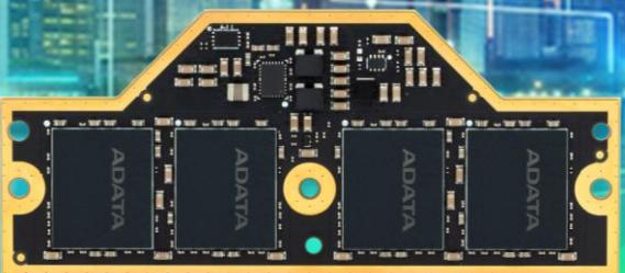
ADATA's LPCAMM2 redefines high-performance embedded memory with an ultra-slim, single-sided form factor. The module enhances signal integrity with simplified motherboard routing and reduces mounting space by up to 60%, allowing greater flexibility for custom cooling and system design.
